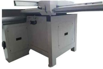
Panel saw fence slides on a precision round bar
